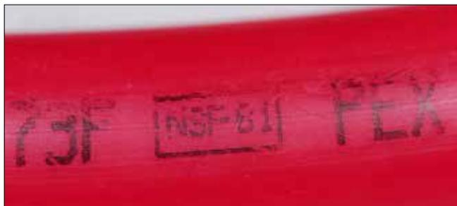
American Boat & Yacht Council (ABYC) and National Sanitation Foundation (NSF) standards for onboard potable-water systems require that all plumbing be approved to carry drinking water. The two examples of cross-linked polyethylene (PEX) tubing, **left**, carry either the "potable" or "NSF-61" designation, while the reinforced polyvinyl chloride (PVC), **below**, is labeled for potable water.
