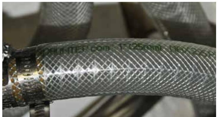
**Left**—While it's commonly installed in onboard water systems, especially by do-it-yourselfers, clear PVC hose is prone to kinking and crushing and should be avoided. **Right**—The exception is kink- and crush-resistant wire-reinforced PVC hose, which is appropriate for pressure and suction applications.
