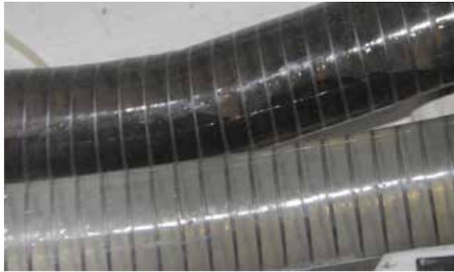
*Potable-water systems, especially those with clear hose, are prone to contamination. The black accumulation inside the top hose doesn't bode well for the quality of the water that passes through it.*
