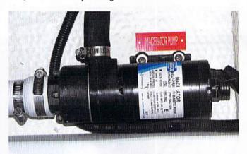
All parts of the sanitation system through which water or effluent moves must be winterized using nontoxic antifreeze. A portion of the system that is often overlooked is the overboard discharge or macerator pump, such as the one shown here.
