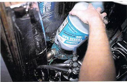
Left: Don't forget to winterize deck washdown pumps, spigots, and strainers. Located in faraway places, these are often overlooked, with dire consequences. Right: Nontox may be poured directly into the raw-water strainer in order to flush the engine as it's running. Don't let the engine run for more than a few seconds without either water or nontox being drawn into the strainer.
