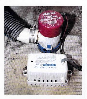
Bilge pumps and their associated plumbing must be flushed with nontox. If water leaks into the bilge during storage and the pump operates, it will need to be re-winterized.
