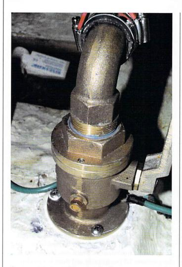
If a seacock is closed while a vessel is afloat, water remains trapped within that seacock. If it is not opened once the vessel is ashore, or drained using a plug, it may freeze and fracture.
