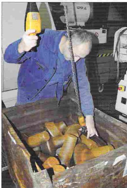
Far left —Toothed gear hobs like this one are ubiquitous in ZF's production facility, where they are employed to cut gears. Left —A technician selects cast blank forms to be machined into finished gears.
