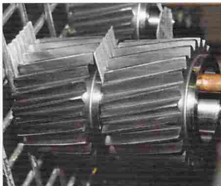
Above —Finished gears are hung on copper rods and separated by aluminum plates. Because both metals are softer than the finished gears, the latter are protected from damage prior to installation. Left —A skilled technician assembles precisely engineered components into a nearly completed transmission.
