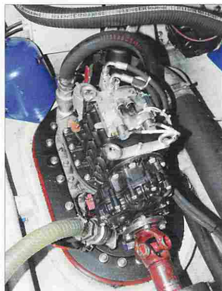
Left —This company test boat exhibited superb maneuverability with fingertip control, two virtues of marrying ZF's pod drives to the company's joystick for low-speed operations. The shift/throttle control is mounted temporarily to ease installation of new models for testing. Right —One of the test boat's two pod drives. The engine is located just forward of the drive, linking to it through the driveshaft and universal joint at the bottom of the photo.
