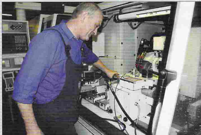
Before running the cutting program for the part, a technician fixes a roughly shaped metal gearbox pinion into a CNC milling machine.
