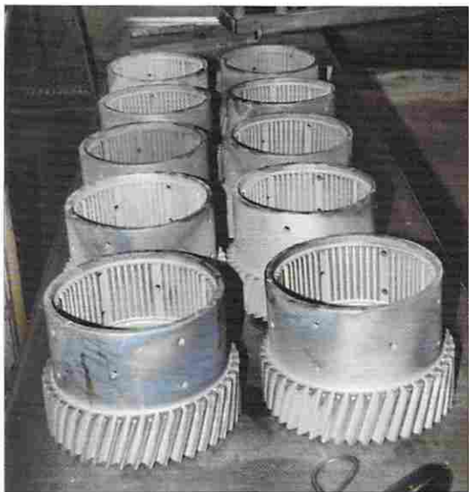
Left —Newly machined gears have been heat-treated in the oven, right , and quenched in a liquid bath to harden them. Next, they are reheated in the oven to a lower temperature to reduce brittleness imparted by the abrupt cooling.
