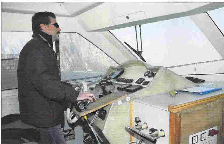
Left —This company test boat exhibited superb maneuverability with fingertip control, two virtues of marrying ZF's pod drives to the company's joystick for low-speed operations. The shift/throttle control is mounted temporarily to ease installation of new models for testing. Right —One of the test boat's two pod drives. The engine is located just forward of the drive, linking to it through the driveshaft and universal joint at the bottom of the photo.
