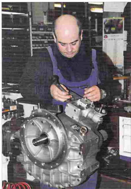
Above —Finished gears are hung on copper rods and separated by aluminum plates. Because both metals are softer than the finished gears, the latter are protected from damage prior to installation. Left —A skilled technician assembles precisely engineered components into a nearly completed transmission.
