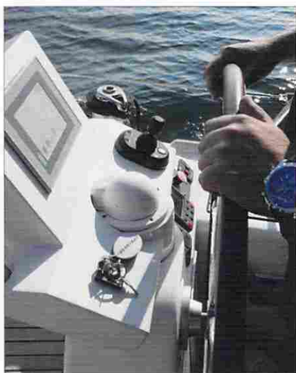
Left —The helm of a Beneteau sloop fitted with ZF's Hybrid SailDrive. Note the joystick control, which allows the helmsman to power the boat sideways or turn in virtually its own length when navigating tight channels and mooring situations, as seen at right , or when operating in a strong crosswind.
