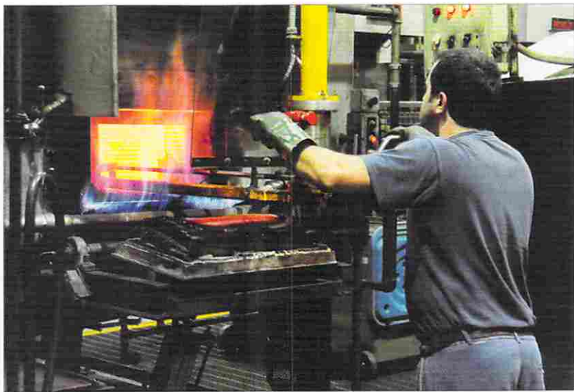
Left —Newly machined gears have been heat-treated in the oven, right , and quenched in a liquid bath to harden them. Next, they are reheated in the oven to a lower temperature to reduce brittleness imparted by the abrupt cooling.
