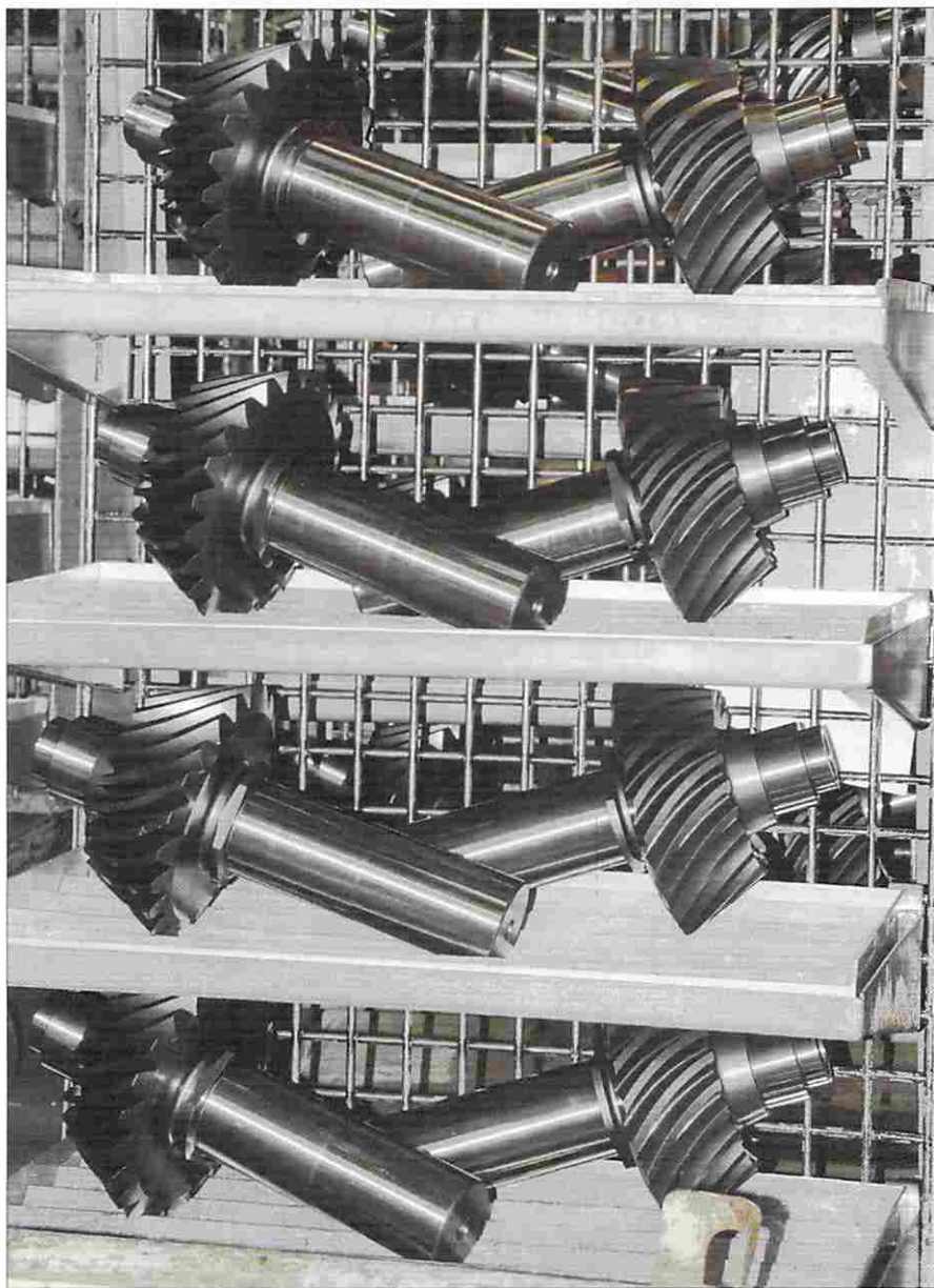
Racks of finely machined and hardened spiral bevel gears await installation at the marine division production facility of engineering giant ZF Marine, in Padua, Italy. The company's initials stand for Zahnradfabrik, "gear manufacturer" in German, and Friedrichshafen, the city in which ZF was founded in 1915.
