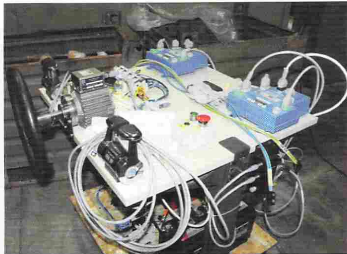
Left —ZF builds transmissions to be fitted to specific models from numerous engine manufacturers. This pallet of six transmissions is bound for Volvo Penta. Right —The SmartCommand control system test platform is composed of a mock-up of networked electronic steering and twin-screw shift and throttle-control systems.
