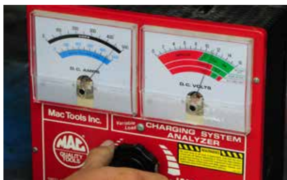
A carbon pile load tester may be used to determine the health of large, deep cycle batteries. By placing a high resistive load on the battery, and then monitoring its voltage and current draw, an accurate analysis of the battery's condition can be determined.
