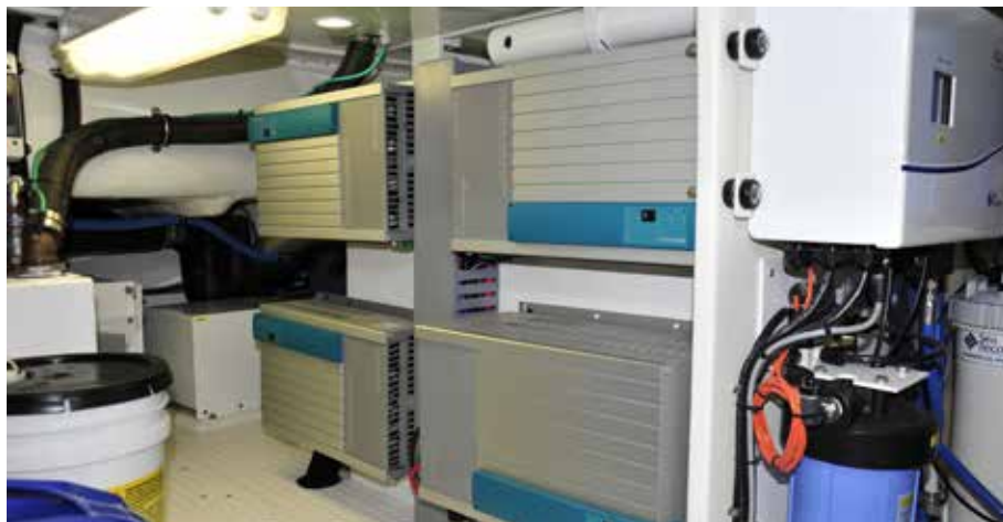
Once unheard of, large, multi-bank inverters have become considerably more common in the past five years. Their output can be equal to that of a medium-size generator. When linked to appropriately sized alternators, they are capable of powering air conditioning systems, ranges and other high current consumers without the need to start, or add wear and tear to, a generator.
