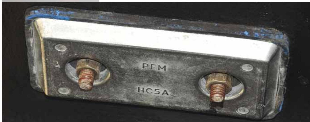
Below: Aluminum anodes, like the one shown here, offer a variety of advantages, including increased amp hour capacity and functionality in fresh, salt and brackish water.
