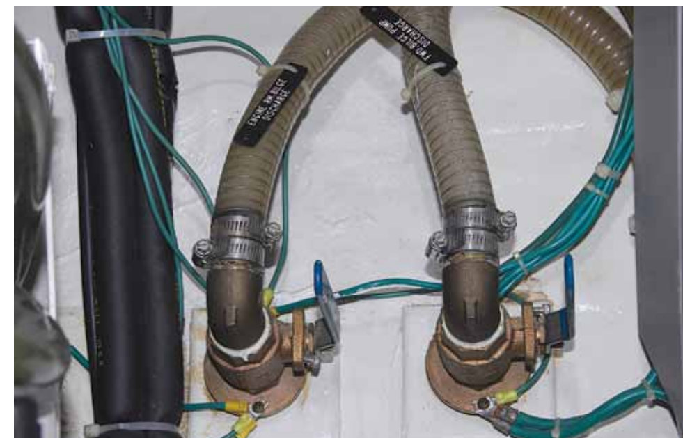
Left: Underwater hardware should bond in such a way as to avoid using the fittings as the current path. The fittings in this image are incorrectly wired. Right: Galvanic isolators are an inexpensive means of preventing shore-ground wire-induced corrosion. Units should be fail-safe and comply with the latest ABYC standards.
