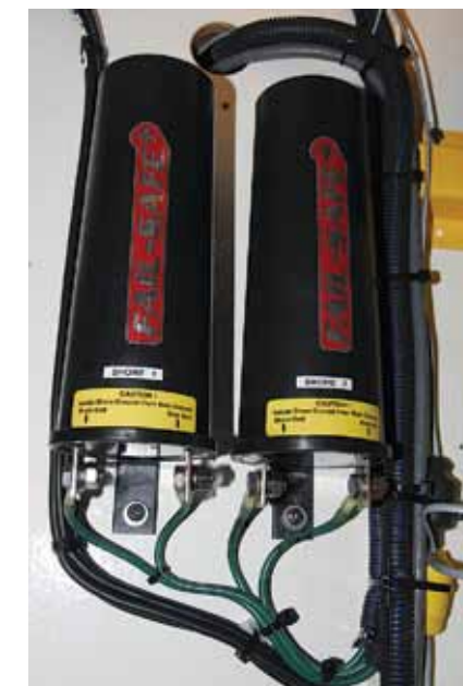
Left: Underwater hardware should bond in such a way as to avoid using the fittings as the current path. The fittings in this image are incorrectly wired. Right: Galvanic isolators are an inexpensive means of preventing shore-ground wire-induced corrosion. Units should be fail-safe and comply with the latest ABYC standards.
