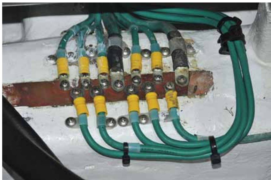
Using tapping screws, screwed into wood or fiberglass virtually guarantees a poor connection; it's also a violation of ABYC guidelines.
