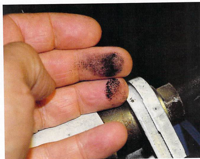
Excessive, rapid accumulation of belt dust is often an indication of misalignment of a component or automatic tensioner.
