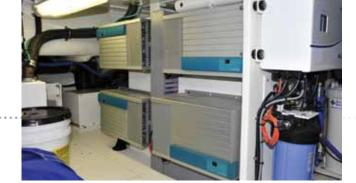
Today, very large inverter "banks"—this one is 15kW—can provide generator-like power for a vessel, provided the battery bank and charge sources are up to the task.
