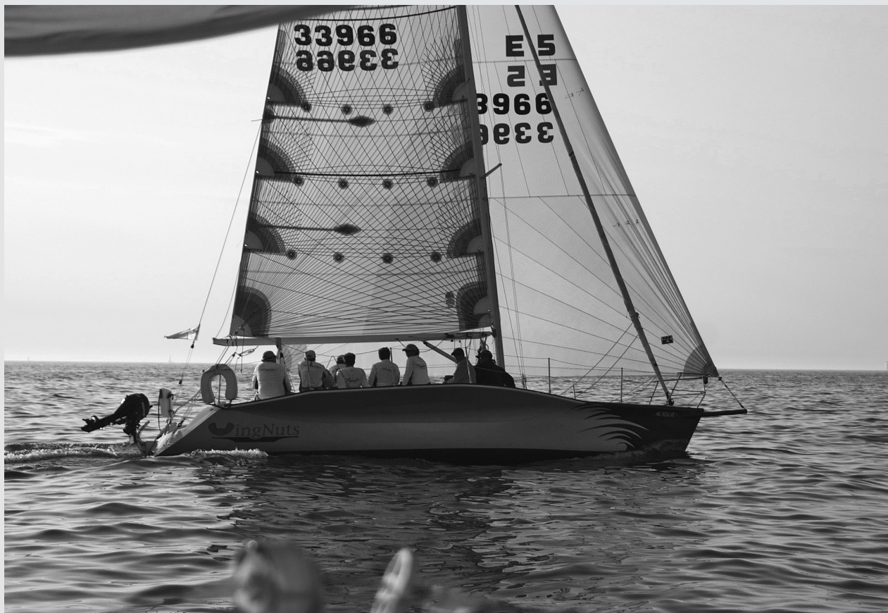
▀ WingNuts under sail. Vessel design was a major factor in her capsize when a fast-moving thunderstorm overtook the fleet of the 2011 Chicago Mackinac Race. Note the wide deck with minimal corresponding hull volume beneath. This design characteristic emphasizes the need for movable crew ballast, rather than buoyancy-induced form stability. The net result is a precipitous drop off in righting moment at angles less than 80 degrees—just when it is needed most. (See Chapter 12 for a fuller discussion of stability and vessel design.) (Courtesy Hubert Cartier)
