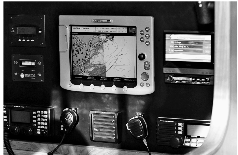
Most manufacturers of network-capable multifunction displays offer a satellite weather service that can display forecasts, GRIB files, and other useful weather information.
