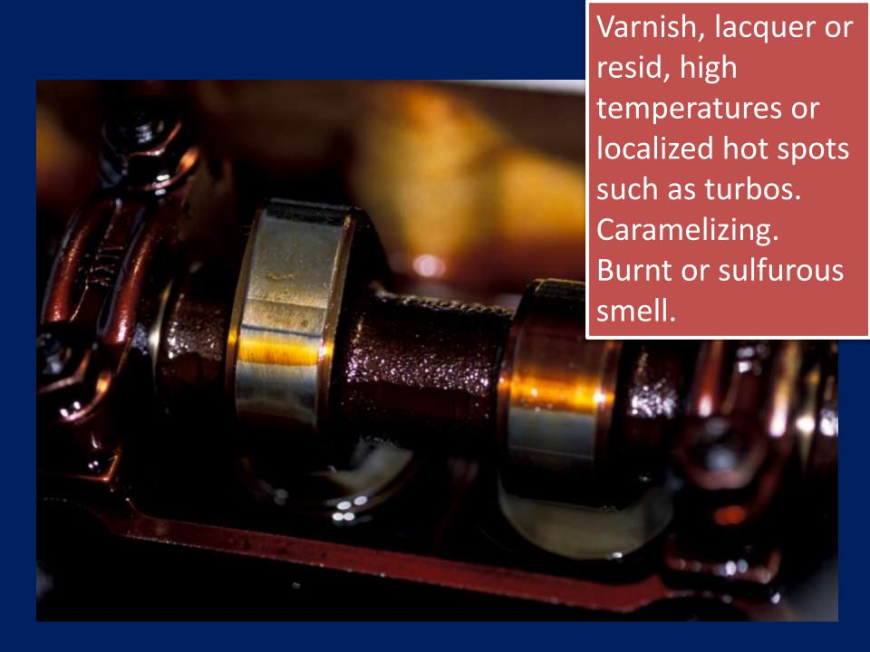
Causes for sludge and varnish can be identified using analysis. Can lead to oil starvation and abrasion.
