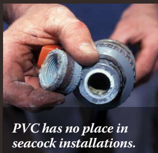
Brass threads in a raw-water discharge after only a year.
