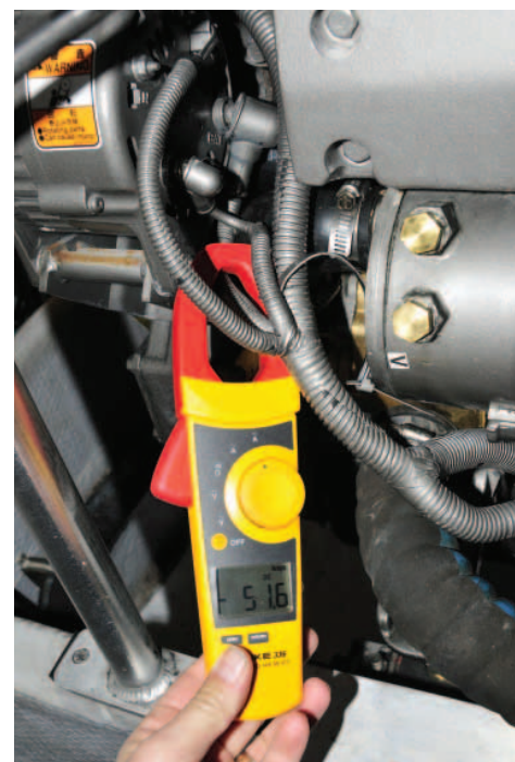
Clockwise from top left: All types of engine instrumentation offer valuable information; Tools such as a digital multimeter are an essential part of any sea trial—make sure alternator output is tested with the vessel's battery charger off; Fluid analysis, it's as close as you can get to a mechanic's crystal ball.
