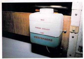
This shouldn't be your only "spare" coolant. Lay in a sufficient supply of coolant in order to deal with a leak. If your engine calls for conventional diluted coolant, consider making up a 50 percent solution for ready use. Be sure to mark the container as premix and use only distilled water for this application.
