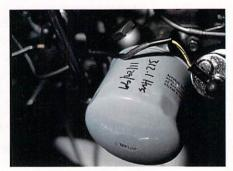
Labeling spin-on oil and fuel filters with date and engine hours of last replacement will serve as a service reminder. This practice will also aid you in determining if and how many replacement elements you will need during a cruise.
