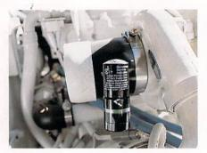
An air filter condition indicator, much like a fuel vacuum gauge, will alert you to a clogged air filter. When resistance in the air filter element exceeds a certain limit, the indicator moves from "GREEN" to "REPLACE" condition.
