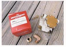
A complete replacement water pump. It's simple: Unbolt the old one, bolt on the new one and you are ready to go. Some engines require removal of other components to access the pump, so assess your situation before counting on this quick fix.
