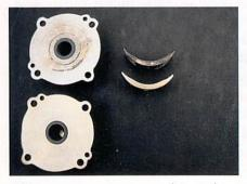
Old raw-water pump cover plate and cam shown at top, spares on the bottom. Notice the degree of wear on the old units. This is sometimes not evident until they are compared to the spare parts. This pump had weak water flow; in comparing the parts it's easy to see why.
