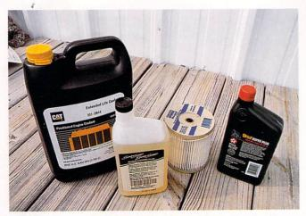
Essential engine fluids and filter, left to right: Specialized coolant that is appropriate for your engine (this is a particular issue for new diesels, which often specify proprietary nonmix coolants), hydraulic fluid for steering system, primary fuel filter element (one is never enough) and crankcase oil.
