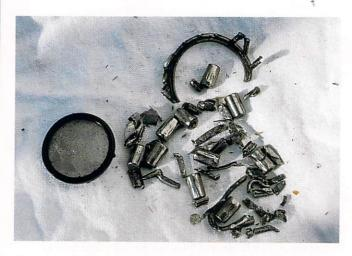
You're not likely to carry spares to resolve this failure. It's probable that the transmission these parts fell out of was destroyed because the wrong fluid was used for lubrication. It's important to carry spare parts and fluids; however, it's more important that they be of the correct type and variety.
