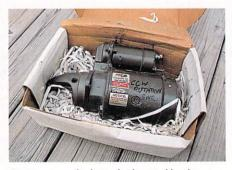
Starts are costly, but rebuilt units like this one are often available at considerable savings. Be prepared to pay a core charge, since you will not be turning an old unit in at the time of purchase. To store, this unit should be sprayed with a corrosion inhibitor, bagged and then replaced in its cushioned box.
