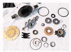
The guts of the average gear-driven raw-water pump. These seemingly simple devices contain a plethora of components. If you are uncomfortable disassembling and reassembling this profusion of parts, you might be better off replacing the pump en masse.
