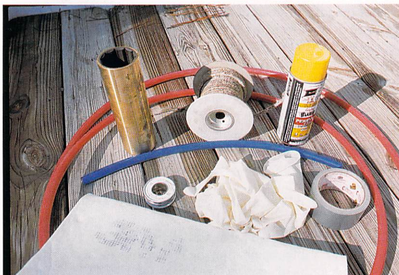
An assortment of spares that may be found in the cruiser's spare parts locker. These include a cutless bearing, flax packing, penetrating lube, seizing wire, rubber gloves, oil absorbent pads and tape.
