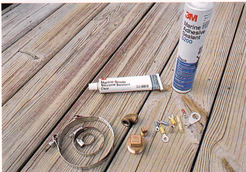
Adhesive, sealant, hose clamps, plumbing fittings and electrical terminals all should have their place in your spare parts locker.
