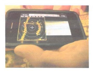
Smart phones with nav apps can be used as remote displays and some can even control what's displayed. Here a radar and a FLIR picture occupy the screen. These very small screen and non-waterproof nav tools are vulnerable to the elements.
