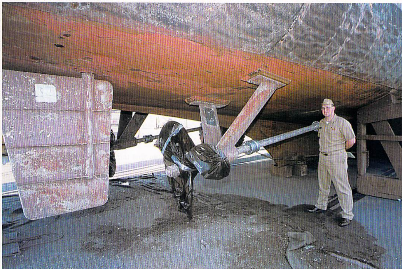
Lt. Denver Applehans, USNR, puts the YP's enormity in perspective as he stands next to the rudder and prop of a YP refit.
