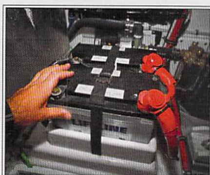
Battery boxes are especially well-suited to flooded battery installations (left); however, the shoebox-like lid must not form an envelope in which hydrogen gas can be captured. Batteries must be secure and completely immobilized, and their positive terminals must be insulated. This installation (center) covers all those bases. A fiddle or frame around a battery bank (right) can serve two purposes: to contain electrolyte and to keep the batteries stable.
