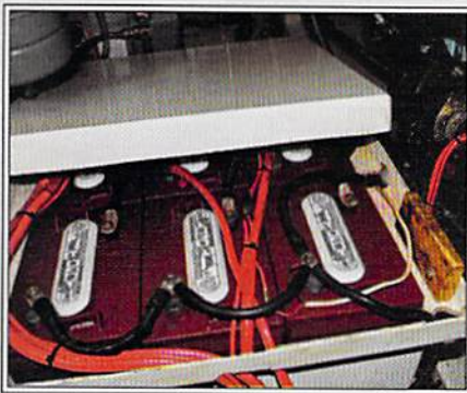
Battery boxes are especially well-suited to flooded battery installations (left); however, the shoebox-like lid must not form an envelope in which hydrogen gas can be captured. Batteries must be secure and completely immobilized, and their positive terminals must be insulated. This installation (center) covers all those bases. A fiddle or frame around a battery bank (right) can serve two purposes: to contain electrolyte and to keep the batteries stable.
