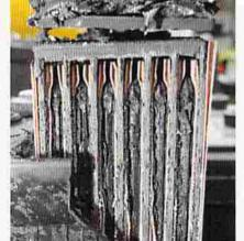
The disemboweled plates of this battery died a premature death from sulfation (left). Large house battery banks that are undercharged or that remain discharged for long periods often suffer loss of capacity through sulfation (top right). Some batteries can be salvaged through a process called equalization using a constant-volt and -current shop charger (bottom right).
