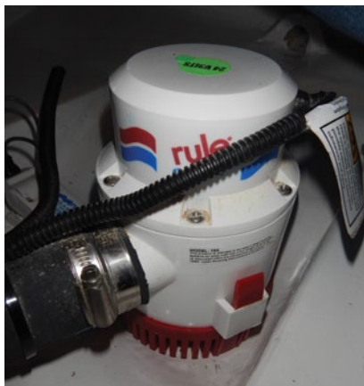
Motor loads like bilge pumps have slightly different overcurrent protection needs. The OCP must also protect a motor that has locked, preventing overheating and a possible fire.
