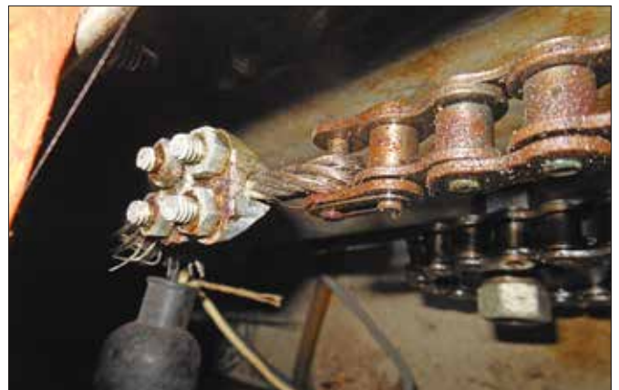
Left —Wire rope, or “bulldog,” clamps must be installed in only one orientation, with the “live,” or tensioned, portion of the cable retained in the clamp saddle, as illustrated here. Right —A cable should never be joined to a chain or quadrant without the benefit of a thimble to hold an appropriate radius in the wire and bear any chafe between the working components. Note that wire clamps should be stainless steel. The galvanized mild-steel ones, shown here, are beginning to rust.
