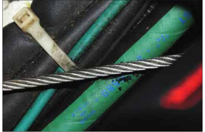
Left —Broken wire strands, or “meat hooks,” are a clear sign that a cable should be replaced. Even one broken strand is too many. Right —Another reason to be particular about leads is that where they unintentionally contact hose, electrical wiring, or wood, steering cables effectively become cutting tools.
