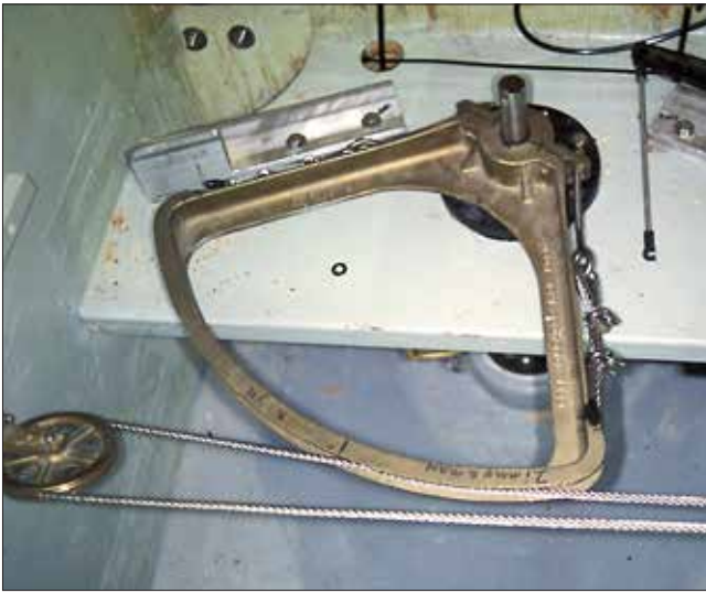
Above left —This standard cable-over-sheave quadrant is partially installed. In service, the quadrant must be protected from any stored items, while being easy to reach for inspection and repair. Above right —The chain-and-sprocket assembly of this cable system runs close to multiple electrical components, which must be secured or physically isolated to prevent chafe. Right —This cable-over-sheave chain succumbed to crevice corrosion that grew from microcracking caused by the stresses of neglect or overtensioning. Thoroughly grease chains and sprockets, and every few years wash them in solvent such as kerosene before renewing the grease.
