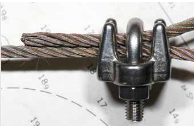
Left —Wire rope, or “bulldog,” clamps must be installed in only one orientation, with the “live,” or tensioned, portion of the cable retained in the clamp saddle, as illustrated here. Right —A cable should never be joined to a chain or quadrant without the benefit of a thimble to hold an appropriate radius in the wire and bear any chafe between the working components. Note that wire clamps should be stainless steel. The galvanized mild-steel ones, shown here, are beginning to rust.
