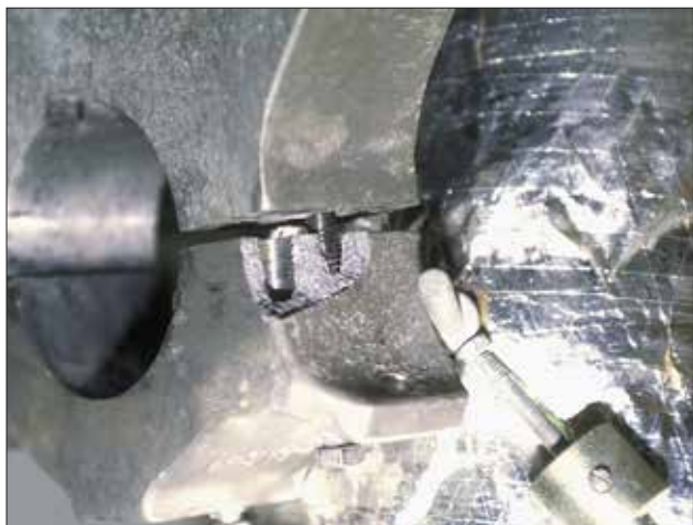
Left —The bore in this radial drive casting was likely undersized for the stock, so it cracked when the clamping fasteners were tensioned. Right —If the design can support them, radial drives offer the potential benefit of eliminating a set of sheaves.
