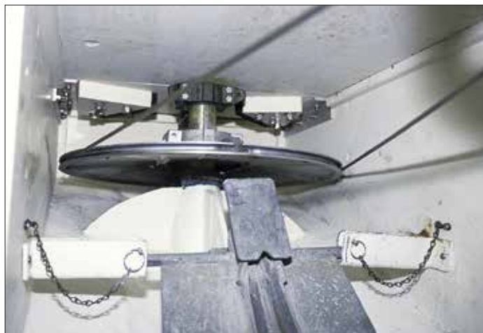
Left —The bore in this radial drive casting was likely undersized for the stock, so it cracked when the clamping fasteners were tensioned. Right —If the design can support them, radial drives offer the potential benefit of eliminating a set of sheaves.
