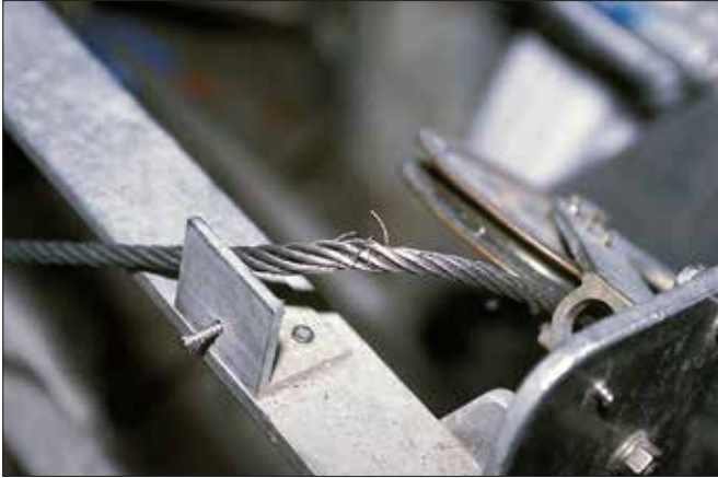
Left —Broken wire strands, or “meat hooks,” are a clear sign that a cable should be replaced. Even one broken strand is too many. Right —Another reason to be particular about leads is that where they unintentionally contact hose, electrical wiring, or wood, steering cables effectively become cutting tools.
