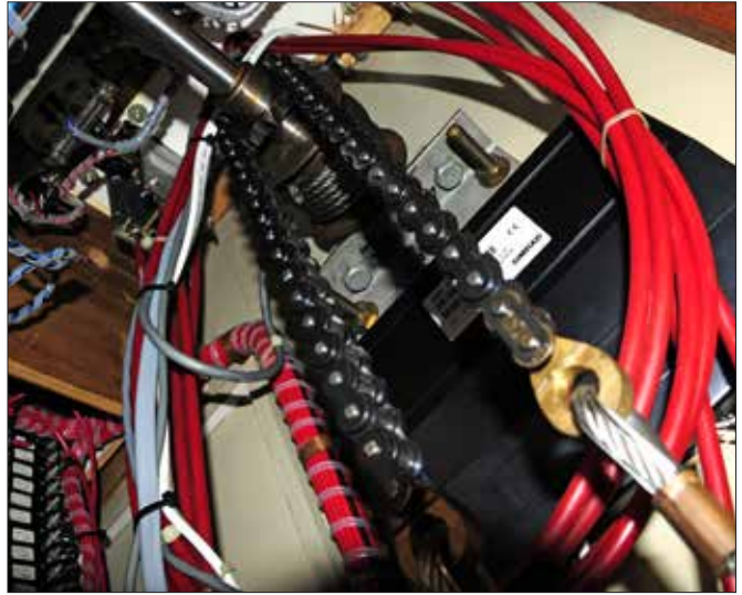
Above left —This standard cable-over-sheave quadrant is partially installed. In service, the quadrant must be protected from any stored items, while being easy to reach for inspection and repair. Above right —The chain-and-sprocket assembly of this cable system runs close to multiple electrical components, which must be secured or physically isolated to prevent chafe. Right —This cable-over-sheave chain succumbed to crevice corrosion that grew from microcracking caused by the stresses of neglect or overtensioning. Thoroughly grease chains and sprockets, and every few years wash them in solvent such as kerosene before renewing the grease.
