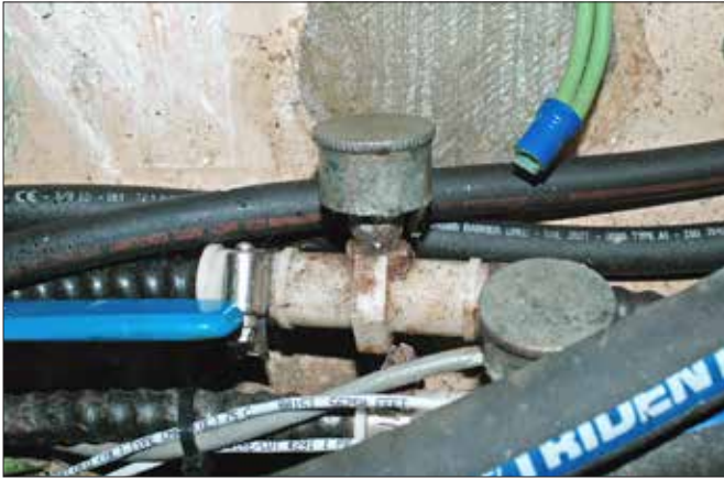
Pull-pull system internal steel cables ride inside a flexible steel jacket. Adequate lubrication to prevent drag and corrosion is essential. Grease cups, like the one shown here, aid in that effort.
