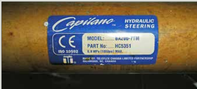
The majority of hydraulic autopilots and manual hydraulic steering systems operate with a relief pressure of 1,000 psi (69 bar). All plumbing components—rams, hoses, and fittings—in these systems must carry this minimum pressure rating.
