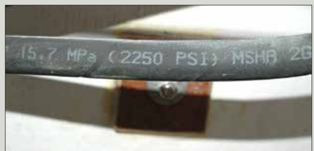
The majority of hydraulic autopilots and manual hydraulic steering systems operate with a relief pressure of 1,000 psi (69 bar). All plumbing components—rams, hoses, and fittings—in these systems must carry this minimum pressure rating.
