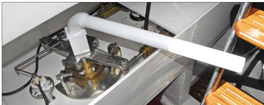
Above —Emergency tillers should be easy to access and fit snugly to the rudderstock. This one installs handily but is a bit short for practical steering. Facing page —Essential to emergency tiller use is the bypass valve (red arrow) that lets fluid circulate in a failed or compromised hydraulic system while allowing the piston to dampen motion.
