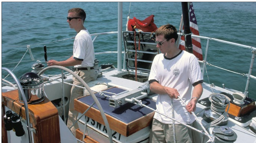
U.S. Naval Academy midshipmen operate an emergency tiller as a training exercise on the 60' (18.3m) Hood-designed sloop American Promise . With good maintenance, the vessel's robust hydraulic steering system proved reliable for 20 years and thousands of miles of hard offshore sailing.
