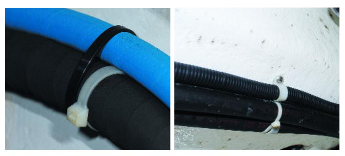
Opposite page: In order to comply with ABYC guidelines, all metallic fuel system components, such as this stainless steel distribution priming manifold, must be connected to the vessel's bonding system. Above left and right: Securing fuel lines by using plastic wire ties is acceptable; however, it should be the exception rather than the rule, and plastic wire ties should never be used in locations where fuel lines pass over machinery with moving parts, such as engines and generators.
