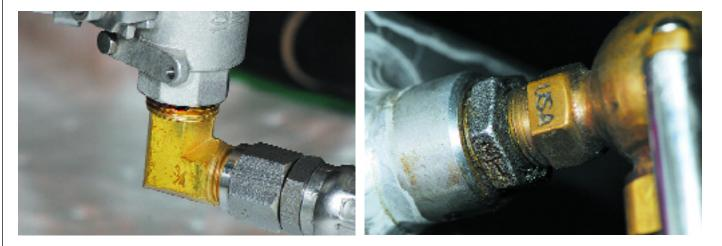
Left: Swaged fittings, such as the one shown on the right, are an alternative to field-attachable hose ends. They are not reusable in that they cannot be detached from the hose once compressed. An advantage is that they are available in stainless steel. Right: Threaded NPT pipe connections are among the least reliable where fuel systems are concerned. Threads should be sealed with a suitable liquid or paste compound such as Loctite 567, 515, or 518.
