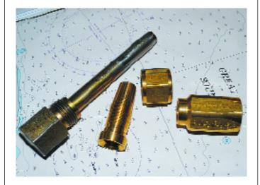
A Parker field-assembled hose connector and the mandrel tool that's used to assemble it. These fittings are extremely durable and reliable and lend themselves to use in boat construction, repair, modification, and service work.
