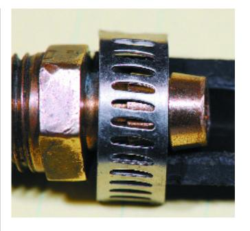
A cutaway view of a hose and barb assembly. It's important to note that the length of this barb prohibits the installation of double clamps.
