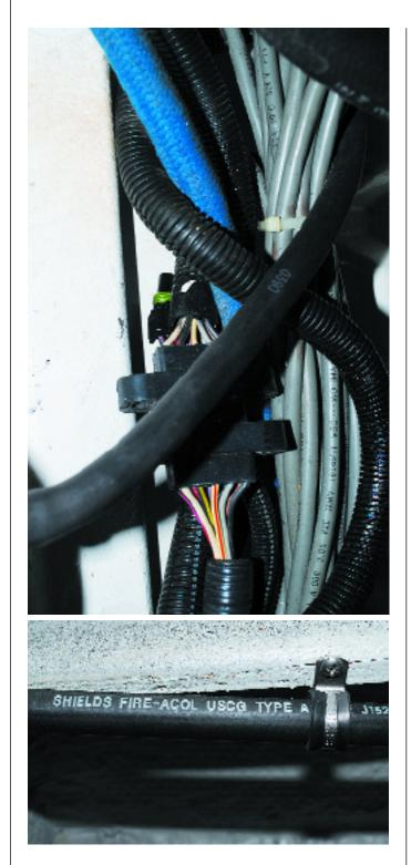
Top: Although bundling or colocating fuel lines with electrical cables, such as those shown here, is not prohibited by ABYC standards, it should be avoided where possible. An electrical short or fire could be exacerbated by burned or melted fuel lines. Above: Insulated metal P clips provide a secure, rugged means of routing fuel lines through machinery spaces. These clips will not degrade when exposed to heat, vibration, ozone, or leaking fuel.
