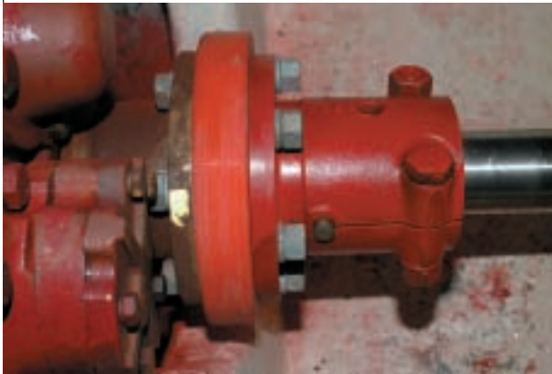
Above left: The clamping bolts on this coupling identify it as one of the split variety. This coupling is also fit with a retaining drift pin, visible at the terminus of the split. These couplings are desirable for their ease of removal from the shaft. Above right: A V-strut whose cutless bearing has been removed. The V configuration is sometimes used for added shaft stability where a longer strut is required. The appendage attached to the left side of the strut in this image is the stationary portion of a Spurs line cutter.
