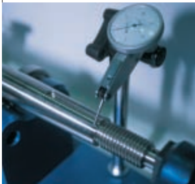
Above left: The tolerance for shaft wear or undersizing is 0.001 inch; any wear beyond that amount condemns the shaft. This shaft is heavily worn where it rode in the cutless bearing, the result of severe misalignment. Right: A dial indicator offers a precision method of determining several shaft faults, including a poor coupling fit or a bent or out-of-round shaft.
