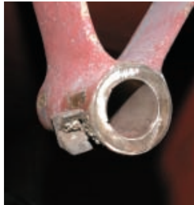
Above left: The clamping bolts on this coupling identify it as one of the split variety. This coupling is also fit with a retaining drift pin, visible at the terminus of the split. These couplings are desirable for their ease of removal from the shaft. Above right: A V-strut whose cutless bearing has been removed. The V configuration is sometimes used for added shaft stability where a longer strut is required. The appendage attached to the left side of the strut in this image is the stationary portion of a Spurs line cutter.
