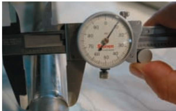
Above left: The tolerance for shaft wear or undersizing is 0.001 inch; any wear beyond that amount condemns the shaft. This shaft is heavily worn where it rode in the cutless bearing, the result of severe misalignment. Right: A dial indicator offers a precision method of determining several shaft faults, including a poor coupling fit or a bent or out-of-round shaft.
