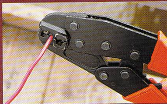
A ratcheting compound (crimps both conductor and strain relief simultaneously) crimping tool.
