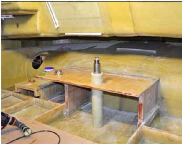
Left —Interior structure is standard plywood pieces tabbed to the hull, including floors and top support for the rudderstock tube. Right —Elling E4's mast, with lights and antennae, hydraulically pivots aft to make the carefully calculated bridge clearances on Europe's canals.
