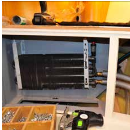
Above —An FRP pan is installed over the glassed-in wood floors, with cutouts for tank access. Right —The hydronic heating-system air handler is installed in a saloon cabinet.
