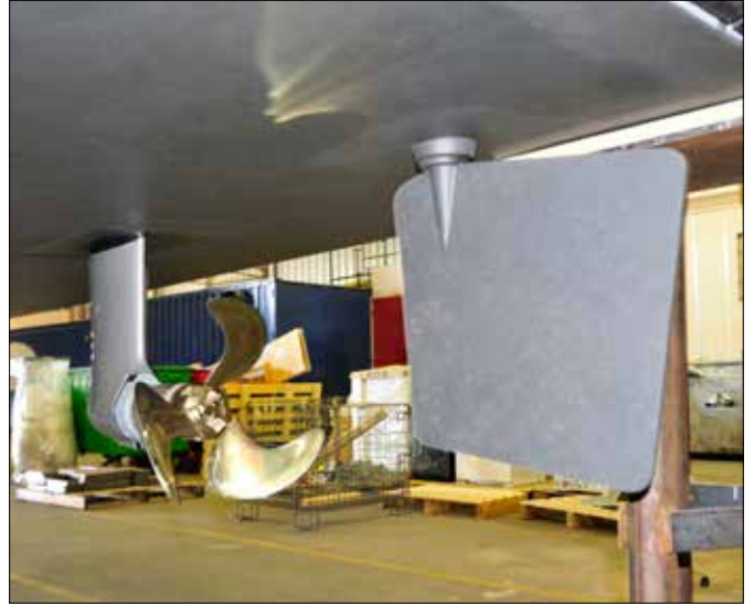
Left —Running gear: skeg-supported propeller shaft, rudder, and externally mounted stern thruster. Right —A popular option for the single-screw motoryacht is a wing engine coupled to a sail drive unit, which of course requires its own rudder for steerage.
