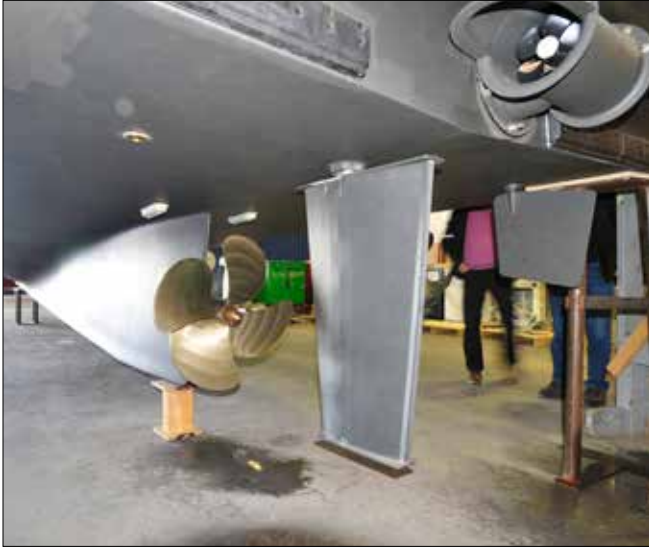
Left —Running gear: skeg-supported propeller shaft, rudder, and externally mounted stern thruster. Right —A popular option for the single-screw motoryacht is a wing engine coupled to a sail drive unit, which of course requires its own rudder for steerage.
