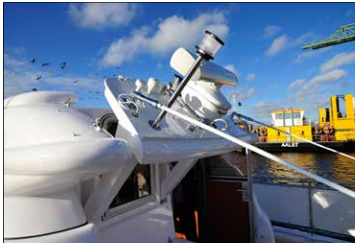
Left —Interior structure is standard plywood pieces tabbed to the hull, including floors and top support for the rudderstock tube. Right —Elling E4's mast, with lights and antennae, hydraulically pivots aft to make the carefully calculated bridge clearances on Europe's canals.
