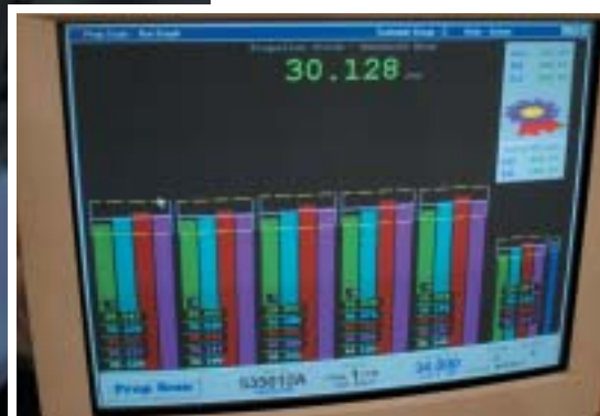
Right: A PropScan bar graph, each color bar represents a different blade, showing the measurements for a propeller that, after being tuned, meets ISO class 1 standards. The dotted rectangle shows the range of acceptable of measurement for this class.
