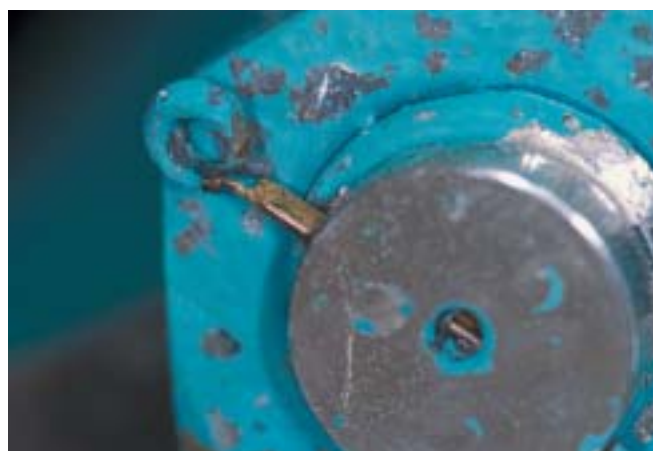
Prop 015: An example of the effects of propeller cavitation. Metal is removed, molecule by molecule, in this process. This propeller is either overpitched, under diameter, lacking in sufficient blade area, or a combination of all three. Prop 016: Propeller shaft cotter pins should always be stainless steel. This brass cotter pin has nearly corroded to the point of failure and it's unlikely it could have retained the nuts and prop in the event that they had loosened. Prop 013: An example of the proper method for installing propeller shaft nuts and a cotter pin. The order of the nuts is important, as is the material used for the cotter pin.
