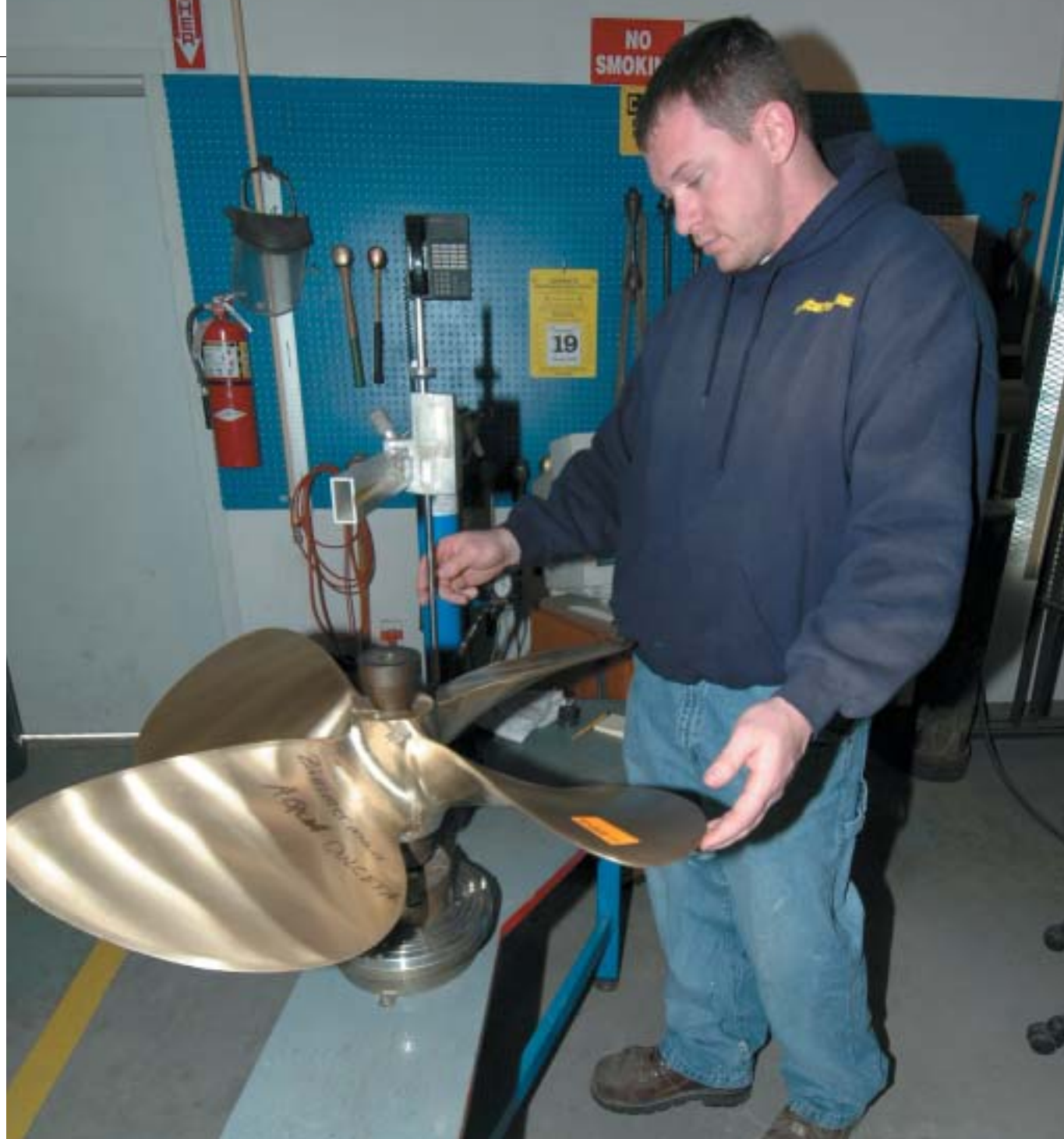
Wildcat Propellers repair technician Troy Erb measures a propeller using the PropScan system.
