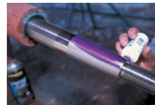
Left: The results of the lapping procedure, the shiny areas indicate contact, where blue remains, however, insufficient contact has been made and thus more lapping is required. Right: Machinist's bluing being applied to a shaft taper in preparation for lapping. Lapping is essential in order to ensure proper shaft taper to propeller bore engagement.
