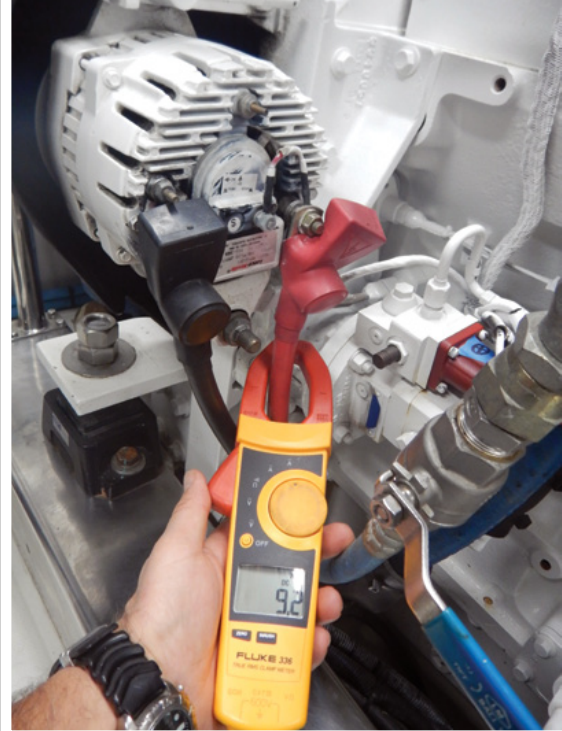
■ The line between hull and engine surveyor can become blurry. Some hull surveyors will, for instance, use a multimeter to assess alternator output, while others consider this the realm of mechanics and engine surveyors.
