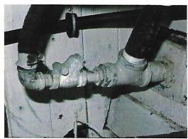
Top left: Plastic through-hull fittings, particularly those that may be located below the heeled waterline, can present a serious liability. A competent surveyor must be able to distinguish between proper and improper plastic or non-metallic through-hull fittings and he or she must understand the difference between a resting and heeled waterline. This through-hull fitting has
