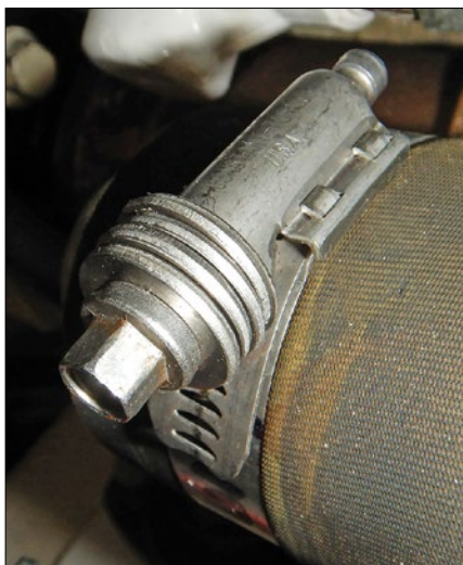
Engines and hydronic heating systems, where heat cycling is an issue, benefit from clamps that can maintain torque as hoses expand and contract. This constant-torque clamp incorporates a spring-loaded tensioner designed to maintain pressure as the hose dimensions fluctuate.
