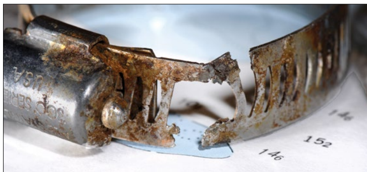
Left —Hose clamps that rely on a perforated thread are susceptible to stress-induced corrosion and failure. Right —Another weakness of perforated hose clamps is their vulnerability to overtightening and thread failure.
