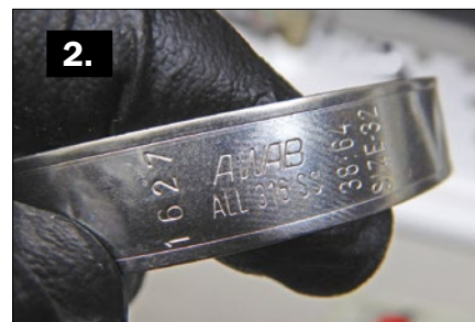
1 —A perforated clamp, left, and a solid-band embossed-thread clamp, right. Not only is the solid band virtually impervious to overtightening and stripping, the thicker metal is less vulnerable to stress cracking. 2 —A clamp marked “all stainless” probably refers to the band and screw. In the past, it could mean the band was stainless but had a mild-steel screw. 3 —The rust-stained bolts on this otherwise good installation illustrate that during manufacturing, it’s not unusual for the stainless steel in fasteners to be converted from highly corrosion resistant to just mildly corrosion resistant (see the sidebar, page 40).
