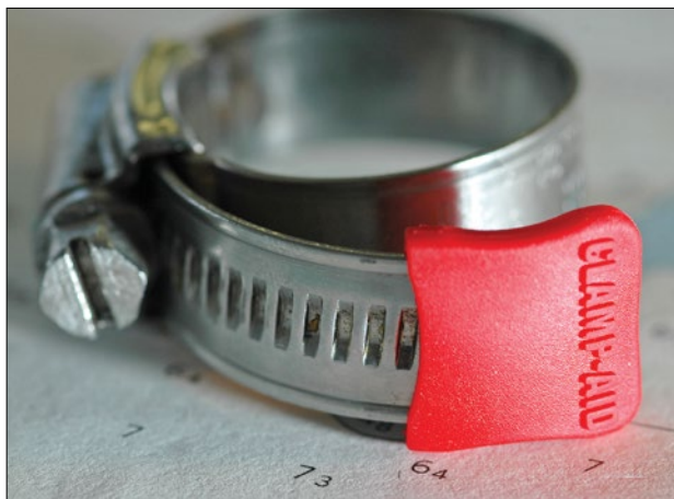
On clamps in high-traffic areas—around engines, and under galley and head sinks—take measures to prevent injury. Left —A proprietary silicone hose-clamp-tail finisher makes the tail safe and is difficult to dislodge. Right —Cap T-bolts with a similar product or, as shown here, a section of appropriately sized hose.
