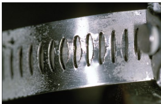
Left —Hose clamps that rely on a perforated thread are susceptible to stress-induced corrosion and failure. Right —Another weakness of perforated hose clamps is their vulnerability to overtightening and thread failure.
