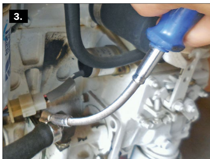
1 —A torque screwdriver is valuable for especially critical applications, or for the inexperienced technician. 2 —A 1/4"-drive socket is perhaps the best tool for tightening multiple clamps. 3 —A flexible hose-clamp drive is the solution where access is challenging. 4 —Common screwdrivers can be used to install hose clamps, as long as the handle provides sufficient purchase to ensure adequate torque is applied.
