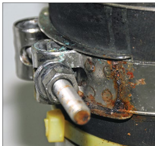
The spot-welded fold in this solid-band clamp is an ideal environment to entrap water, leading to crevice corrosion.
