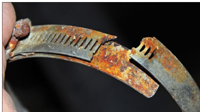
Left —To avoid the undesirable “cheese-grater” effect of overtightened perforated clamps, especially on soft silicone-based hoses, use clamps with embossed, rather than perforated, bands. Above —A clamp variation with a solid band under the perforations protects the hose from the grater effect, but, as shown here, in continuously wet environments it is still vulnerable to microcracking across the band, starting around the perforations.
