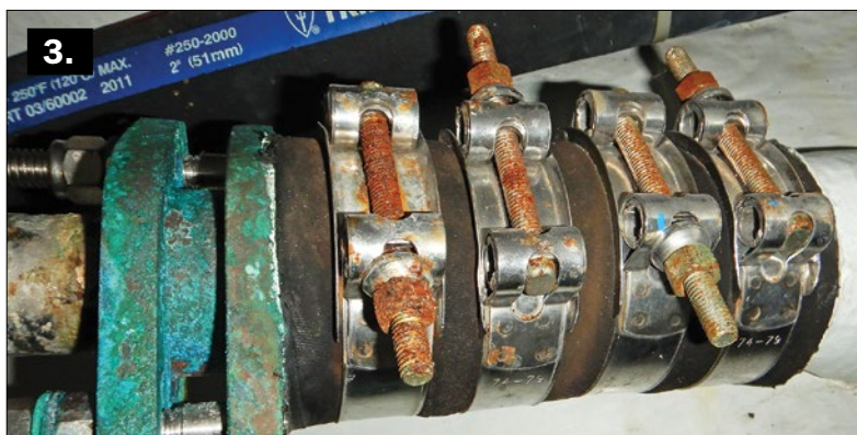
1 —A perforated clamp, left, and a solid-band embossed-thread clamp, right. Not only is the solid band virtually impervious to overtightening and stripping, the thicker metal is less vulnerable to stress cracking. 2 —A clamp marked “all stainless” probably refers to the band and screw. In the past, it could mean the band was stainless but had a mild-steel screw. 3 —The rust-stained bolts on this otherwise good installation illustrate that during manufacturing, it’s not unusual for the stainless steel in fasteners to be converted from highly corrosion resistant to just mildly corrosion resistant (see the sidebar, page 40).
