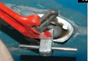
to the portion of the seacock's flange that will be placed against the backing block, being careful to keep sealant at least 1/4" away from the female threads inside the seacock's body. It's important that no sealant be allowed to migrate inside the seacock, where it may impede valve operation.
