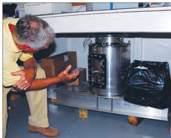
Above —Testing equipment crowds the lab where the myriad challenges of creating a small but sufficiently heavy gyroscope—and the vacuum to spin it in—were overcome.
