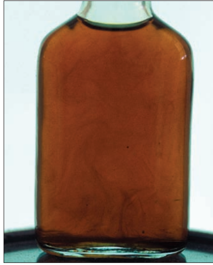
Left —A graphic example of biological growth from a marine fuel tank. Most diesel bio-contamination is bacterial; the lack of light inside a typical fuel tank precludes the ability for algae to exist there. Right —Sampling and inspecting fuel is the most basic way to ascertain its quality. This sample was taken from the tank of a recreational vessel in service for less than a month. Placed in front of a photographer's slide table, the suspended sediment is clearly visible.
