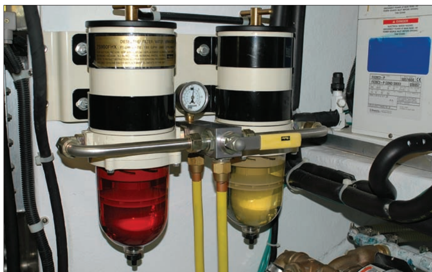
Top —In the U.S., red-dye diesel fuel always indicates untaxed fuel. But, owing to a lack of coordination between federal agencies, the dye can sometimes indicate high sulfur content, too. Worse, different agencies specify different dyes. Bottom —These filter bowls clearly indicate this vessel has taken on two types of fuel: untaxed (or off road) on the left, and taxed (on road, and most likely low sulfur) on the right.
