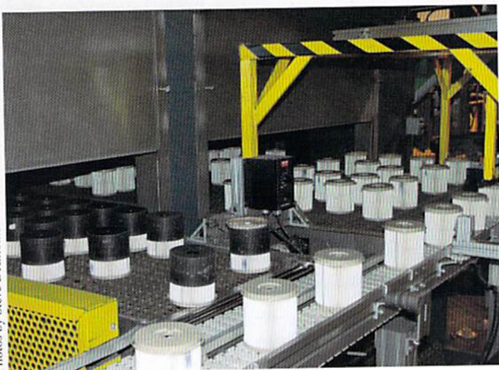
Left: The Modesto facility is capable of making tens of thousands of fuel filter elements each year. Right: Completed marine-series Turbine filters await packaging and shipment.
