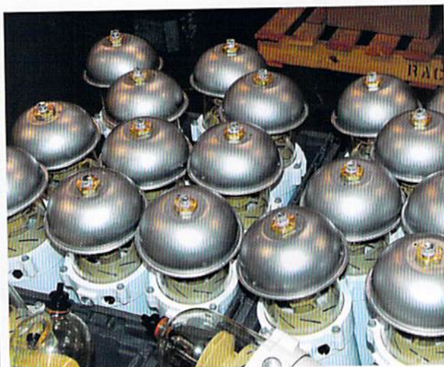
Left: The Modesto facility is capable of making tens of thousands of fuel filter elements each year. Right: Completed marine-series Turbine filters await packaging and shipment.
