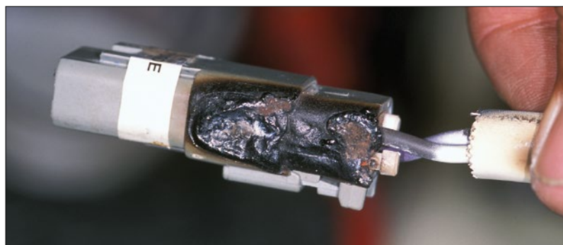
Above —A melted wiring harness illustrates how vulnerable any electrical connection or component is to lightning damage if a boat is not well protected. Right —This unpainted square copper plate on the hull bottom grounds the boat's lightning protection system and satisfies the ABYC guidelines.
