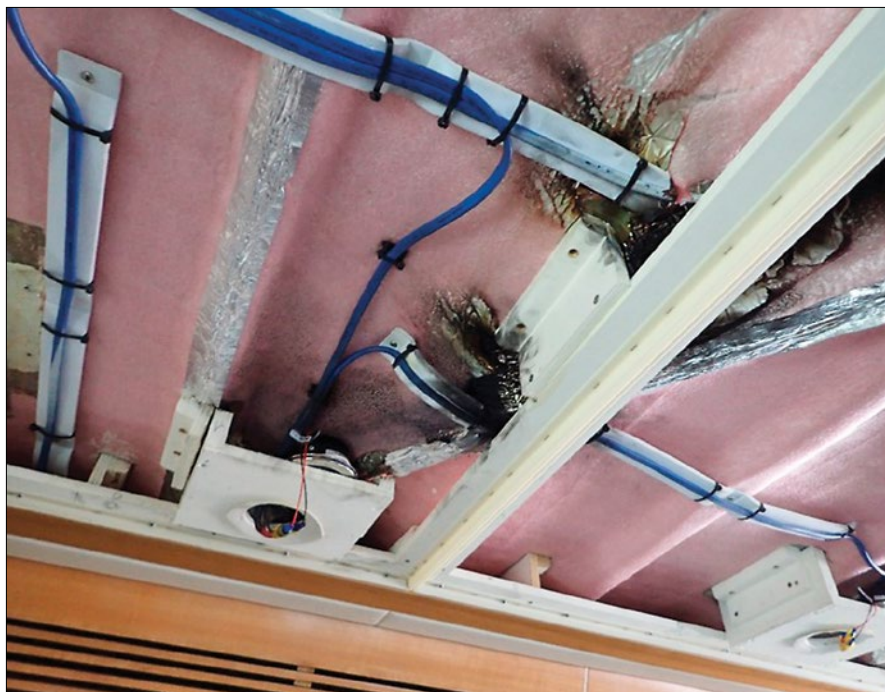
Damage from a lightning strike can play havoc through a boat's electrical system. The overhead in this pilothouse was disassembled to reveal scorching damage along the wiring after a lightning strike.
