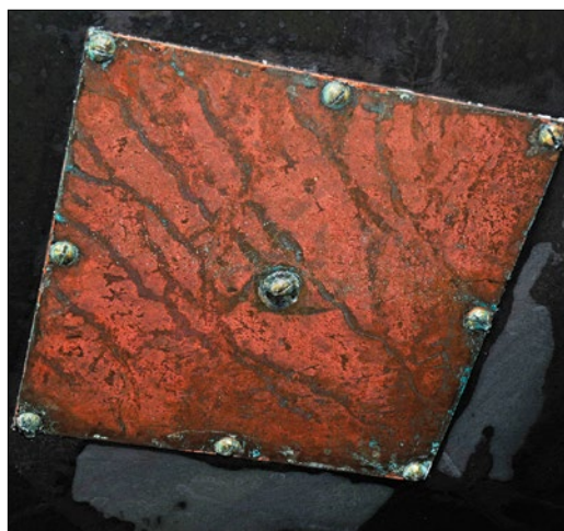
Above —A melted wiring harness illustrates how vulnerable any electrical connection or component is to lightning damage if a boat is not well protected. Right —This unpainted square copper plate on the hull bottom grounds the boat's lightning protection system and satisfies the ABYC guidelines.
