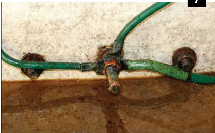
Because the connection to the ground plate is always in the bilge, bonding and lightning systems are especially vulnerable to corrosion, so taking anticorrosion measures is crucial.
