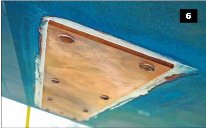
Be sure that bedding compound doesn't obscure the plate's important square edge, while the leading edge should be beveled so lines and objects in the water won't snag on it.
