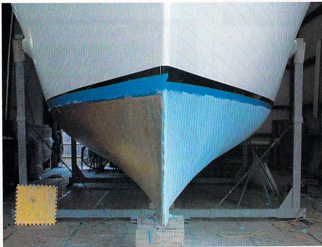
This trawler has had her bottom peeled and relaminated. The blue material seen on the port side is a vinylester fairing compound that improves sandability of the vinylester resin, which makes for an exceptionally smooth bottom. Also, notice the "bottom-free" stands, which support the vessel while the work is being done without interfering with the lamination.
