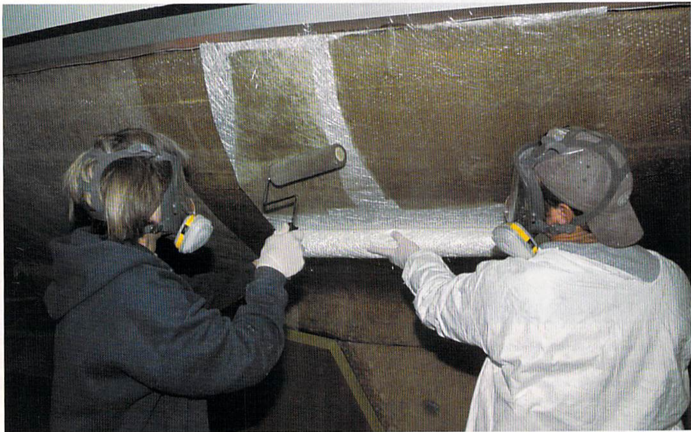
While a skilled pro can make it look easy, the relamination process is often difficult at best, requiring fiberglass technicians to essentially apply resin-soaked fiberglass reinforcement while working upside down.
