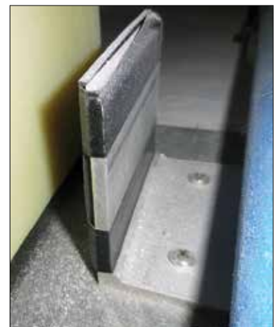
Below —Cross-linked polyethylene tanks undergo one-time expansion when first exposed to fuel; when placing cleats and other supports, that change in size must be taken into account to prevent buckling.
