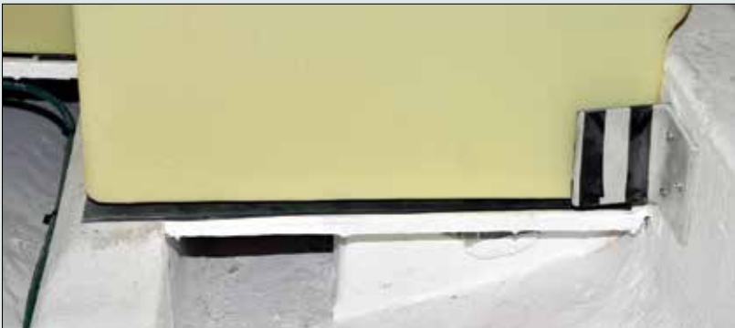
Left —Poly tanks must be supported along their entire bottom panels while also being protected to avoid the potential for chafe. Right —While supporting tanks from above is an acceptable practice, unless specifically designed for it, a tank should not be used to support any structure above it.
