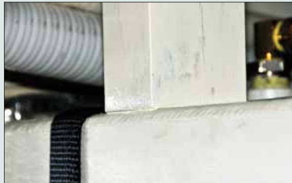
Left —Poly tanks must be supported along their entire bottom panels while also being protected to avoid the potential for chafe. Right —While supporting tanks from above is an acceptable practice, unless specifically designed for it, a tank should not be used to support any structure above it.
