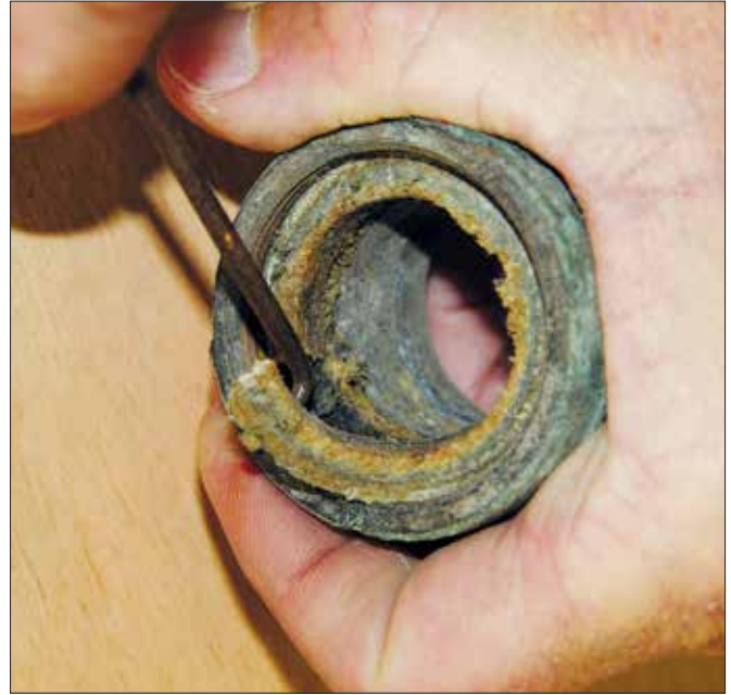
Replace old flax packing material when it loses flexibility and the ability to compress around the spinning propeller shaft in a near-watertight seal.
