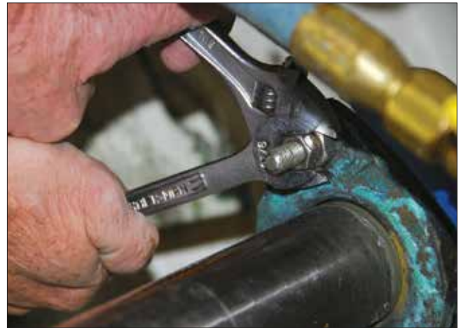
Two wrenches are necessary to properly tighten and lock central, or multiple, tie-rod packing-adjustment nuts.
