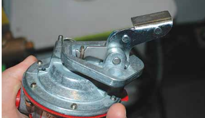
Fuel pumps on many gasoline engines rely on a lever that's driven by the engine's camshaft. Mechanical fuel pumps used on gas engines are different than ordinary fuel lift pumps, in that fuel leaking from within the pump must be captured and sent back to the engine's air intake system, often routed through a clear plastic tube, rather than spilling into the bilge. Check yours to ensure it includes this important safety feature.
