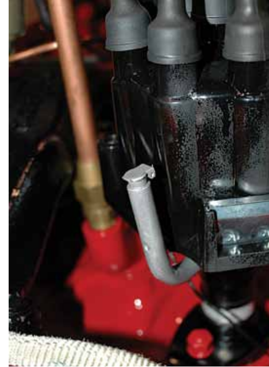
Gasoline engines rely on distributors to send spark to each spark plug and cylinder in a carefully choreographed sequence. However, it's important that, for safety purposes, the inside of the distributor remains isolated to prevent ignition of gasoline fumes.
