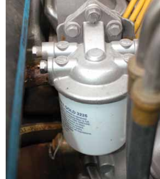
Fuel filters play an important role for any internal combustion engine, and gas engines are no exception. Ideally, the spin on variety, like this one, captures sediment and water.
