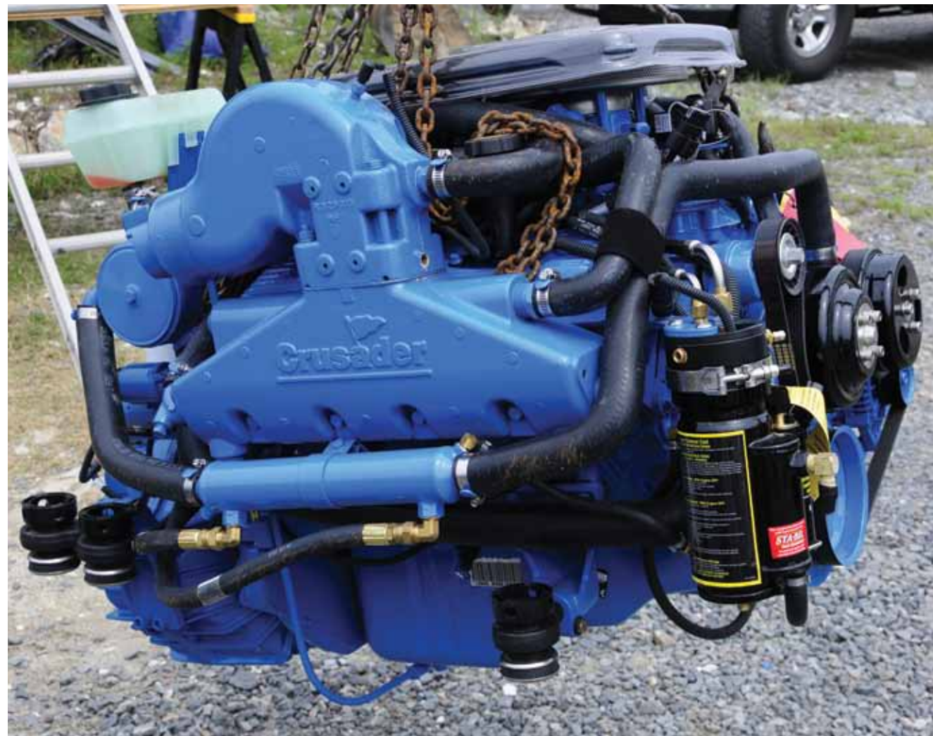
Gasoline engines have a place in propelling cruising powerboats, particularly those that don't accrue significant hours each season.
