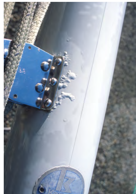
Left—Corners of metal structures are often subject to excessive abrasion and frequently suffer from thin paint coverage making them particularly vulnerable to corrosion. Right—Especially on aluminum spars, paint failures tend to propagate from hardware installations.
