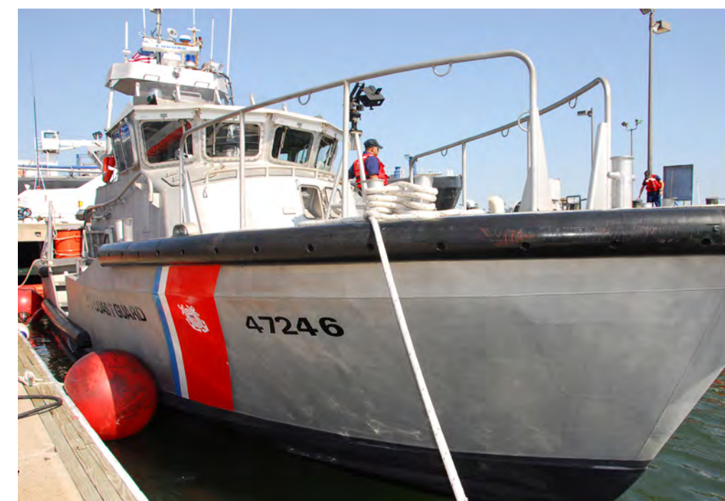
While the metal sits on the vulnerable extreme of the galvanic series, raw aluminum, especially in the 500 or 600 series, is naturally corrosion resistant and used extensively for workboat hulls.
