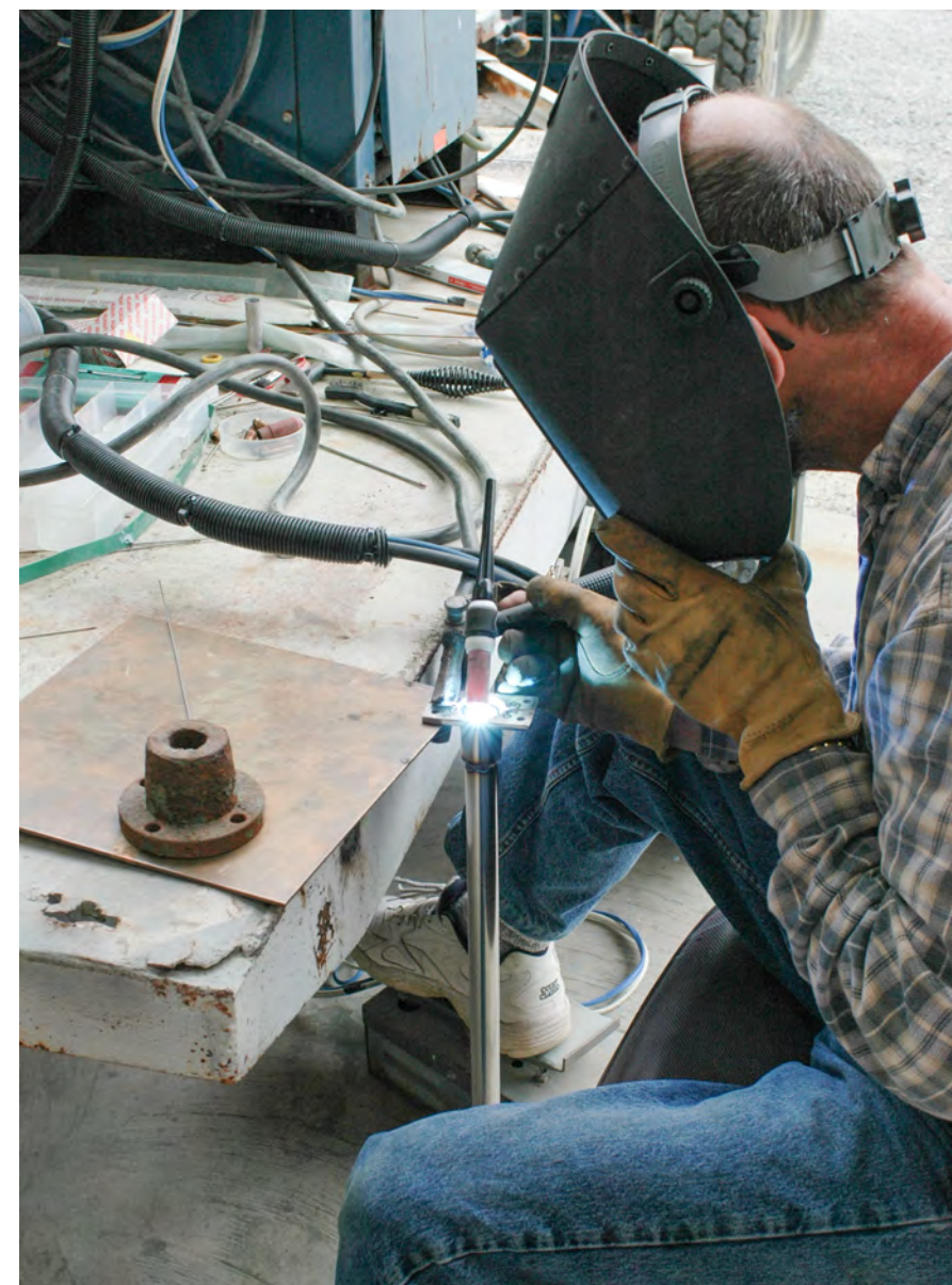
To prevent carbide precipitation, and the corrosion it can facilitate, stainless steel that is to be welded must be of the low-carbon variety, typically identified by an L suffix, such as 304L or 316L.
