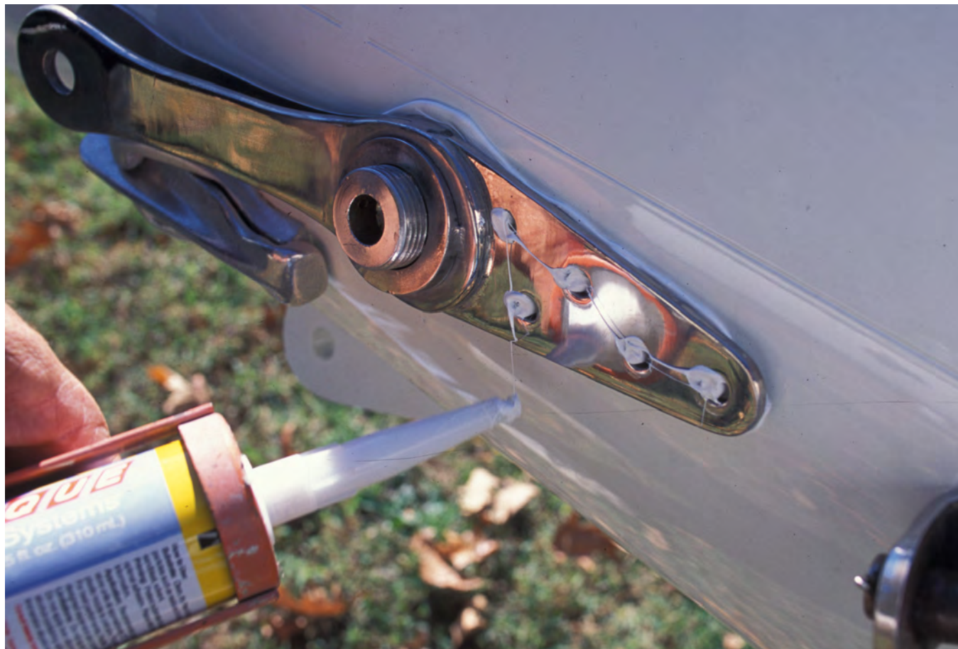
After cleaning painted spar and mounted component surfaces, bedding hardware and fasteners in durable sealant minimizes the risk of paint failure and metal corrosion.
