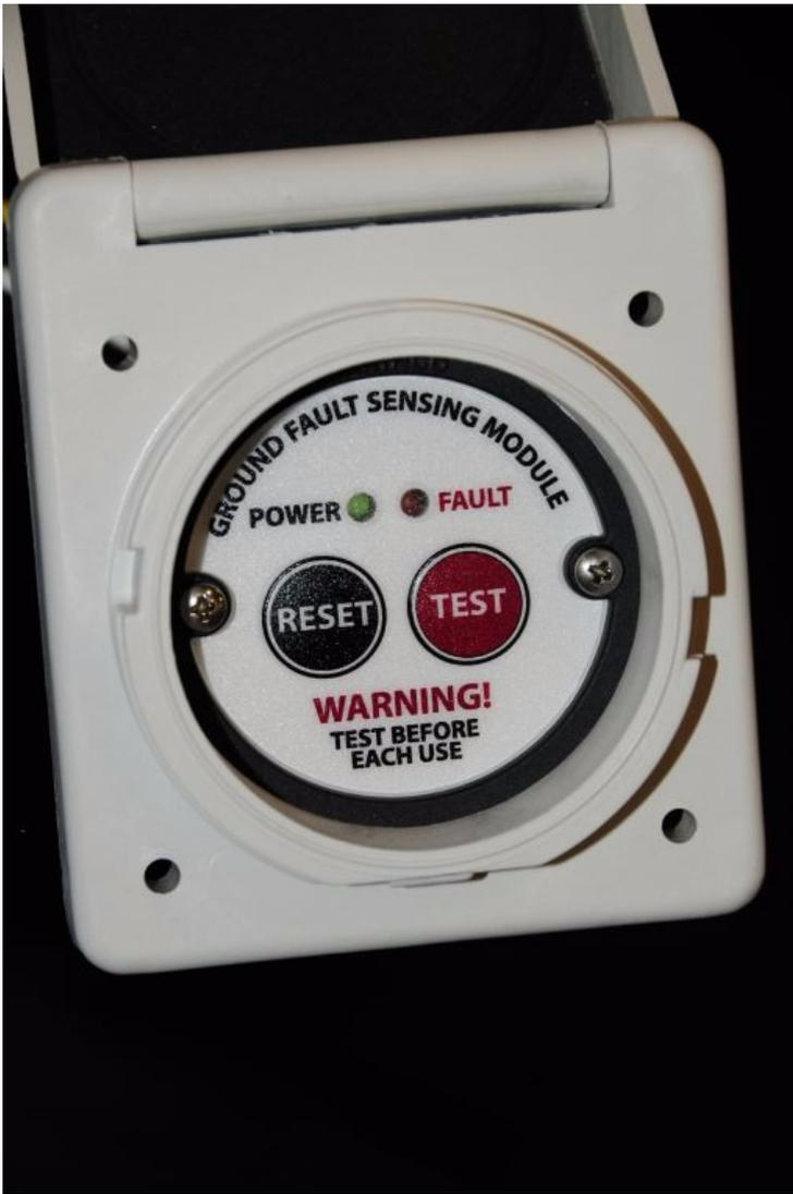
**An equipment leakage circuit interrupter or ELCI, is capable of sensing faults in a vessel's AC electrical system, whereupon it will turn off power in the blink of an eye, ideally before an injury or fire can occur. With few exceptions, ABYC and CE-compliant vessels must be equipped with this component.**
