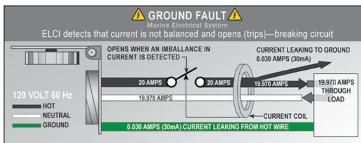
However, if electricity 'leaks' from this intended path in these two wires to ground, this condition is called a ground fault. A good example of this is an insulation failure in the wiring of an appliance.
