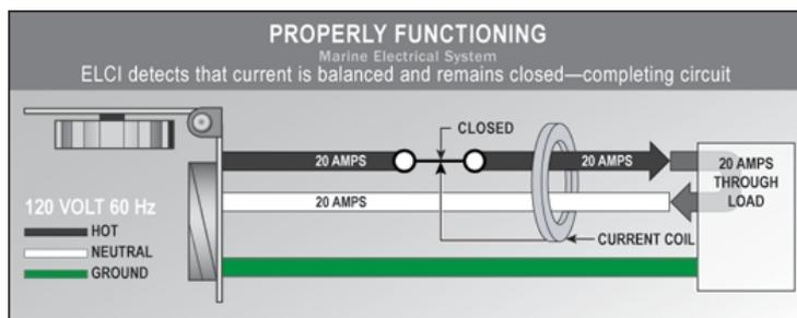
In a properly functioning marine electrical system, the same amount of AC current flows in the hot and neutral wires.
