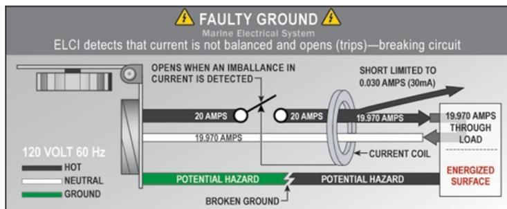
In addition, a faulty ground can occur when the grounding path is broken through a loose connection or broken wire. For instance, a shore power cord ground wire may fail due to constant motion and stress.
